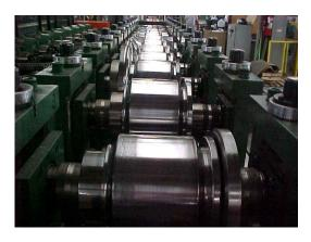
**Roll forming machines** fabricate specific configurations out of long strips of metal, most commonly coiled steel. In most applications, the required cross-section profile of the piece is specifically designed for the machine to bend the metal as necessary. Other than roll forming, these machines perform a number of metalworking duties, including material cutting and roll punching.
