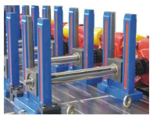
In many modern roll forming machines, programmable logic controllers ensure accuracy. This is vital if a part needs multiple holes or needs to be cut to a specific length. The programmable logic controllers tighten tolerance levels and minimize accuracy.
